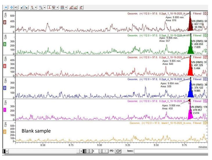
Example of geosmin detection at 0.2 ng/L by optimized HS-SPME-GC-EI-MS/MS (PAL LSI, Bruker TQ). Accredited method (ISO 17025).
